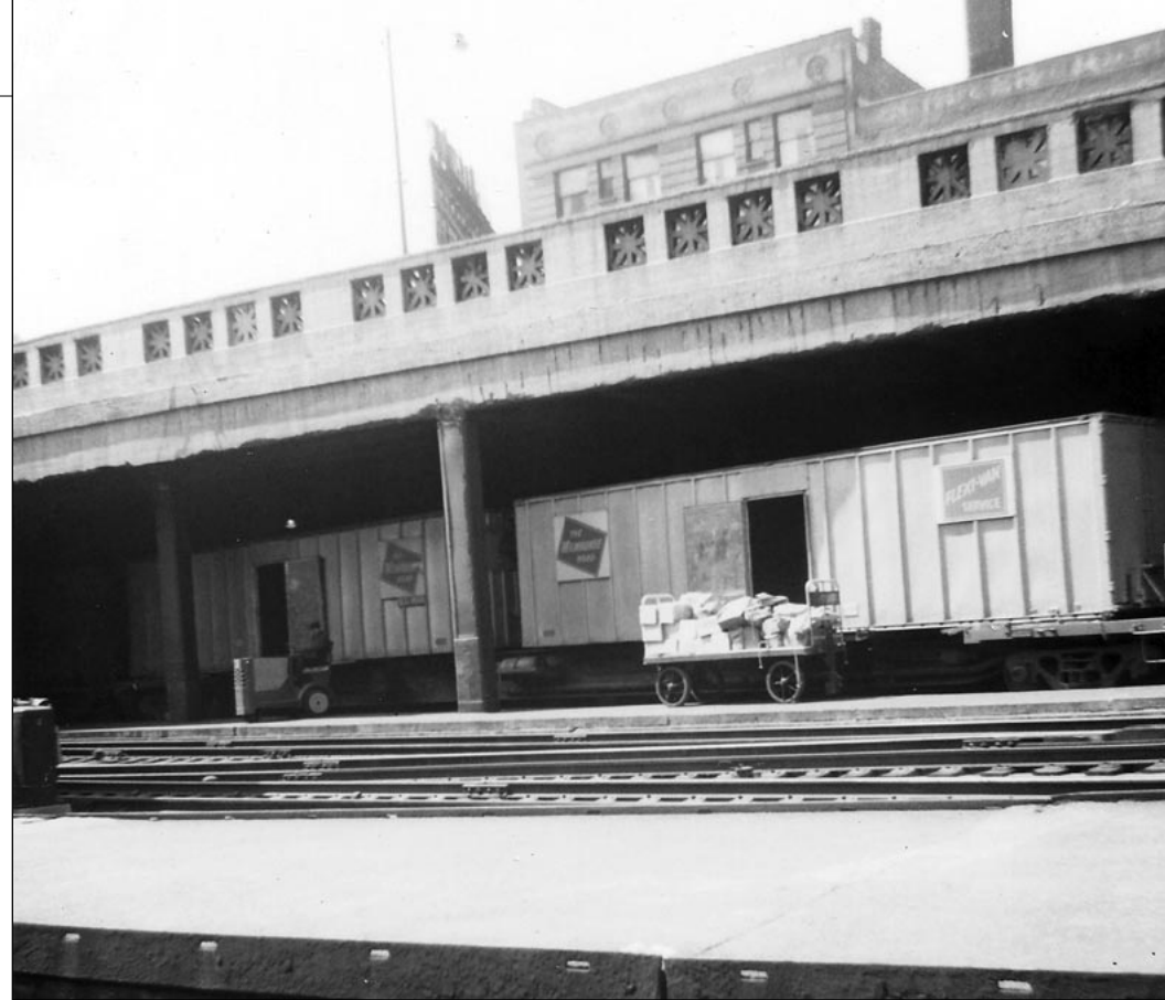
▲ The Milwaukee Road along with the Illinois Central and New York Central were among the few railroads that used the Flexi-Van technology to haul mail and express shipments. Two Flexi-Vans are being unloaded at Chicago Union Station.— Author's photo
