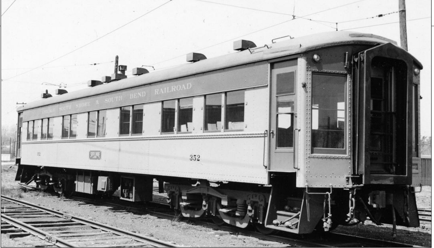
The two parlor cars and two dining cars built by Pullman and delivered in early 1927 were equipped with six-wheel trucks. ▲ Car 352 is at Shops circa 1938.—George Krambles photo, Krambles-Peterson Archive
