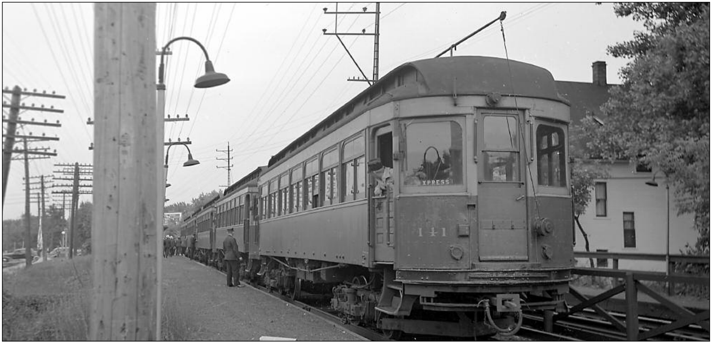
Wooden cars built for both the Chicago & Milwaukee Electric (North Shore Line) and the AE&C served Glen Ellyn. ▲ Car 141 is leading a westbound train of "North Shore Woods" in June 1938. While these cars tended to "nose" on both the North Shore and CA&E, they rode pretty well on the CA&E, due in part, that they did not operate as fast as the CA&E cars. Thus, they tended to be assigned near the ends of the rush hours so as not to delay following trains. ▼ Car 307 is operating solo on a westbound Wheaton local in June 1939. —Two photos Frank Krejcik, Walter Keevil Collection
