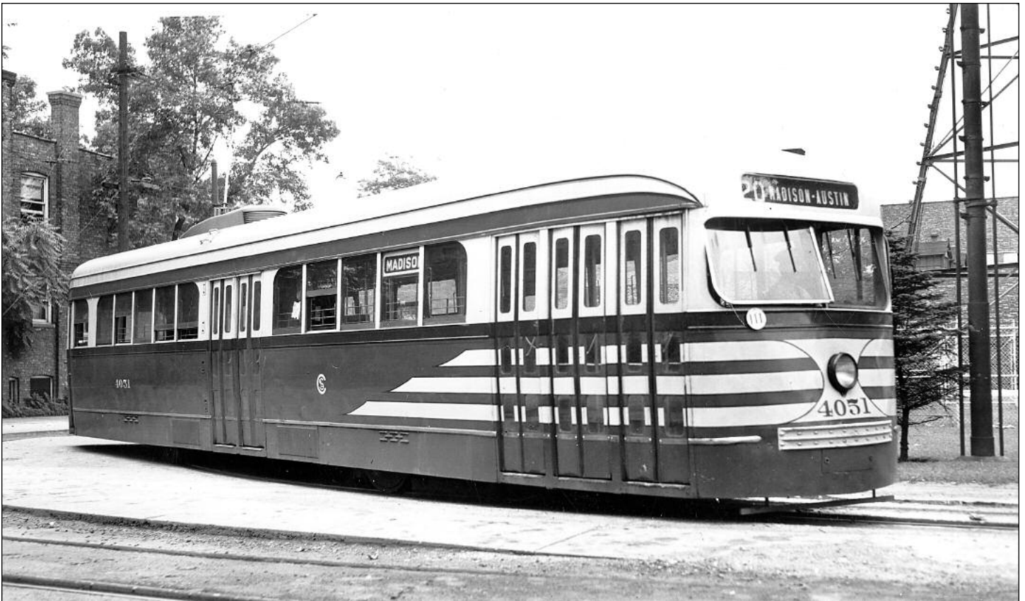
▲ 4051, as rebuilt back to original door layout, prepares for a trip from the west city limits at Madison Street and Austin Avenue to Downtown Chicago. The "tiger stripes" were applied to the car in 1945. — Joe L. Diaz photo, Author's Collection
