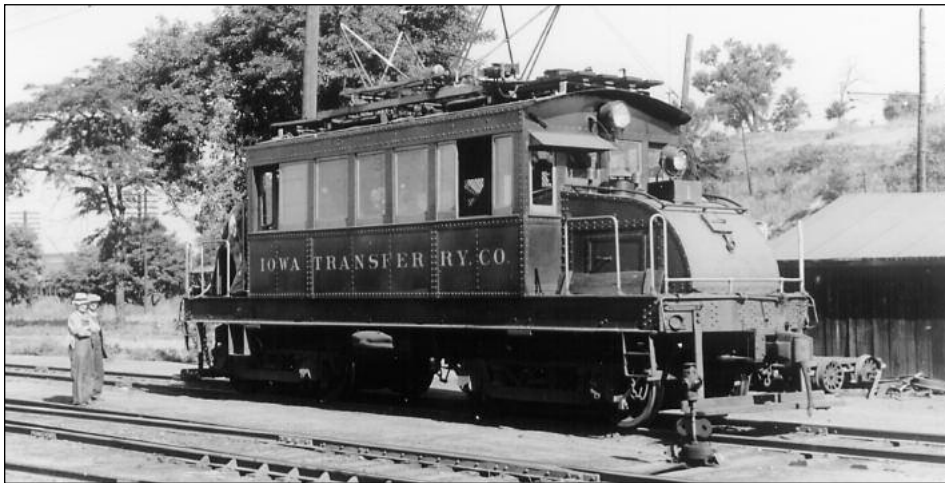
▲ The Iowa Transfer Railway was essentially a joint facility operated for the benefit of its owners and connecting railroads providing yard and interchange services in downtown Des Moines. It was electrified in the interest of smoke abatement. Its sole locomotive was formerly WCF&N 180. Electric operation ended in 1950 when the overhead wire system needed considerable work. Diesel operations ended in 1970 when the owning roads began to operate the yard themselves. —Blair Foulds photo, Norman Carlson Collection
