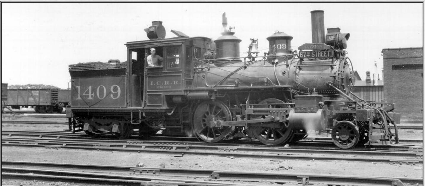
Locomotive 1409 is a part of Illinois Central's initial fleet designed exclusively for suburban service. Some mainline engines have been converted to tank-type locomotives to supplement the fleet as passenger traffic grew. American-type (4-4-0) locomotives are assigned to the suburban service to haul the heavier and longer distance trains that operated to Matteson where higher speeds are involved. *Illinois Central photo, Norman Carlson collection*
