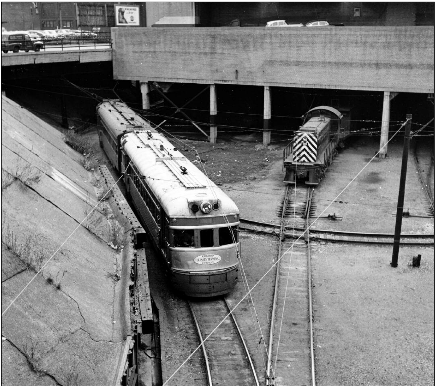
▲ At St. Louis the Streamliner could also not be turned as a trainset. In January 1955, Alco S-2 number 710 is switching the underground freight house. After being wyeed separately, this two-car consist is backing into a station track in preparation for its 5:00 p.m. departure to East Peoria as train 94. —William D. Middleton photo, Norman Carlson Collection
